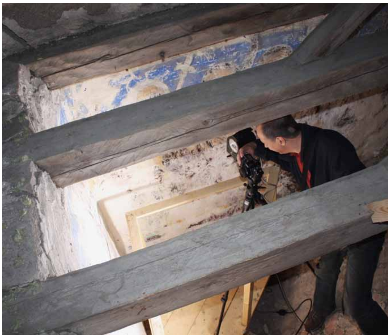
Photographing at site for creation of scale true photo base maps (photo A. Henningsson)
